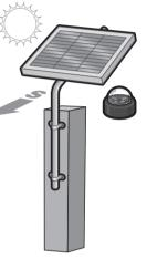
**IMPORTANT:** the solar panel must be positioned facing the path of the sun, due south and in an open area away from shade. It should receive at least 8 hours of direct sunlight for a full charge.
